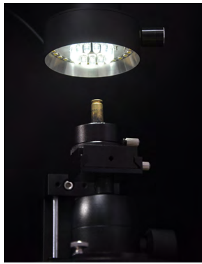
The external coaxial LED ring light is more conducive to the observation of the smooth surface, high reflective and hard-to-reach areas. It contains 13 coaxial lamp beads.
