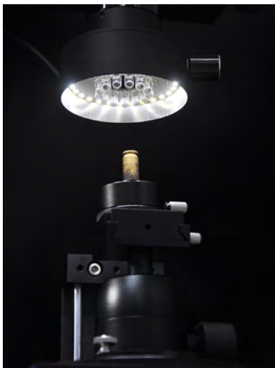
Diffuse emission LED ring lights to reduce glare. Contains 27 diffuse light beads.
