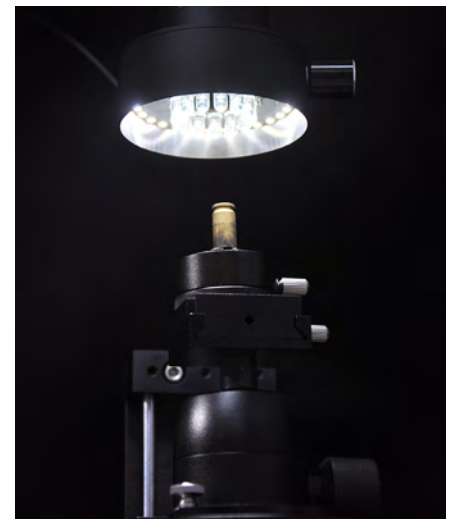
The two ring lights are independently controlled, and the brightness can be freely combined and adjusted according to actual observation conditions.
